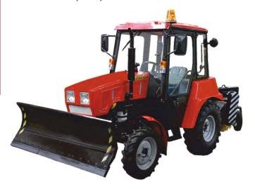
The cleansing vehicle is designed to clean streets, squares, roads and sidewalks from freshly fallen snow and debris, to level bulk soil and fill trenches and pits with it.
