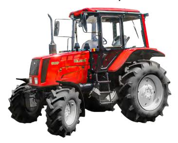
The tractor is intended for the mechanization of rice cultivation, as well as for performing various work in agriculture in combination with mounted, semi-mounted, trailed machines and implements. Distinctive features include increased ground clearance and all-terrain tires. The 920R4 package includes air conditioning.
