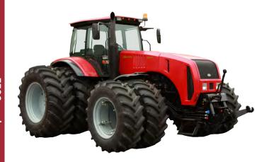
The 3525 tractors are intended for power-consuming agricultural operations in traction and traction-drive modes as part of wide-range and combined units, including arranged in echelon, during primary and pre-sowing tillage, sowing of grains and other crops, forage conservation, harvesting root crops, grains and industrial crops; for hauling operations, stationary work, in construction and industry.
