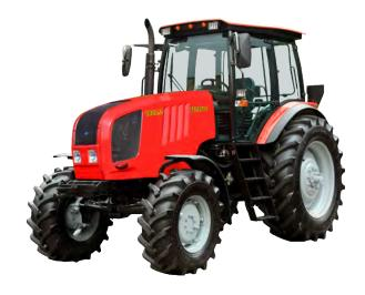
The 1822.3 tractors are intended for various general-purpose agricultural operations, for primary and pre-sowing tillage, for sowing as part of wide-range and combined units, for harvesting operations as part of high-performance harvesting complexes, and for hauling operations.
