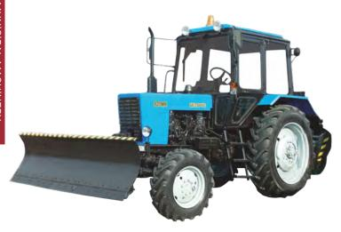
The machine is designed to clear streets, squares, roads and sidewalks with hard surfaces from debris and fresh snow, to shape loose bulk soil and fill trenches and pits with it. The machine consists of a BELARUS 82.1 base tractor and a plow-brush equipment.
