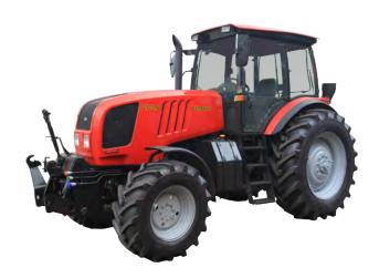
The 2122.3/2122.4 tractors are intended for power-consuming agricultural operations in traction and traction-drive modes as part of wide-range and combined units, including with implements arranged in echelon, and for hauling operations.
