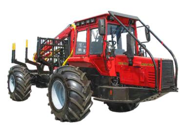
The machine is designed for collecting, loading, transporting assortment along felling sites and skid roads, as well as for unloading, sorting and stacking.
