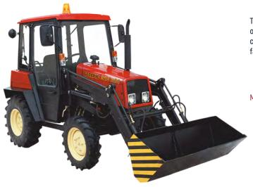
The loading machine is designed to perform material handling operations for site planning, filling trenches with bulk soil, and cleaning roads, sidewalks and areas from debris and freshly fallen snow.
