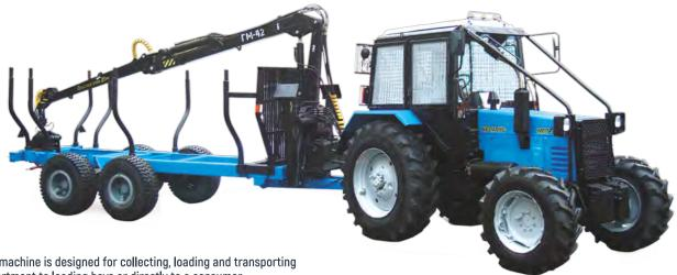
The machine is designed for collecting, loading and transporting assortment to loading bays or directly to a consumer.
