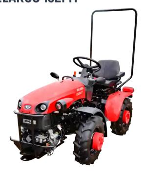
The BELARUS 132MT compact tractor is designed for plowing light soils, harrowing, tilling, inter-row cultivation of potatoes and beets, haying, transporting goods, for stationary work driven by a power take-off shaft, as well as for use in orchards and vegetable gardens, household plots, etc. The tractor is equipped with hydrostatic steering, which makes it possible to operate the tractor more comfortably and with less effort.
