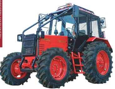
The machine is designed for reforestation and caring for a felling area after deforestation, as well as for collecting, loading-unloading and transporting of assortment, cleaning of felling residues, etc., when using attachments and trailed equipment.
