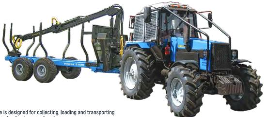
The machine is designed for collecting, loading and transporting assortment to loading bays or directly to a consumer.
