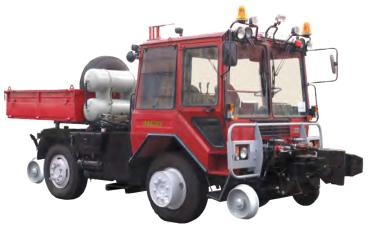
The universal machine is designed for use as a locomotive for shunting operations on in-plant railway tracks with a gauge of 1520 mm, as well as for year-round maintenance and cleaning of public roads, and improvement of industrial areas.
