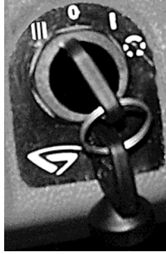
Figure 1.2 – Switch of starter and instruments
